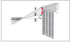
e.g. determining the height between point 1 and point 2 using three target points.
