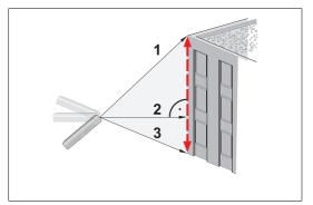
Aim at the upper point (1) and trigger the measurement. After the first measurement the value is adopted. Keep the instrument as horizontal as possible
