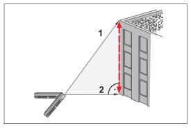
e.g. for measuring building heights or widths. It is helpful to use a tripod when measuring heights that require the measurement of two or three measurements.
